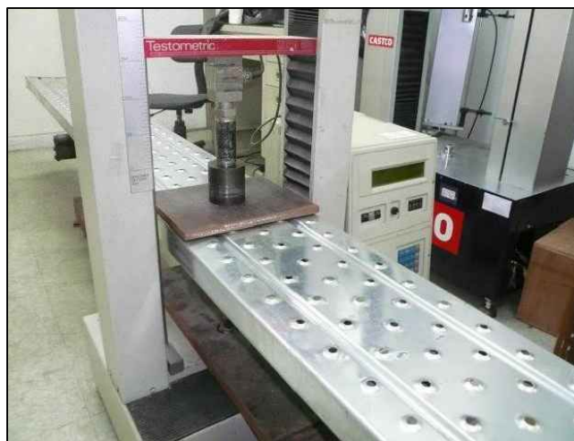
Testing of Planks at Support Interval 1,829 mm, Maximum Load P: 419 kg at deflection 62.02 mm
