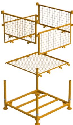
Exploded View of Mesh Box Stillage.
