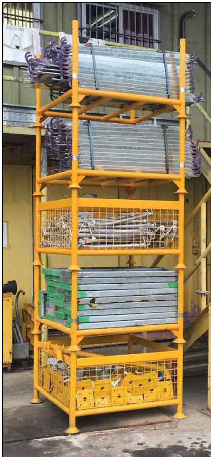
Sample stacking of various types of post stillages storing scaffold components of different types and sizes.
