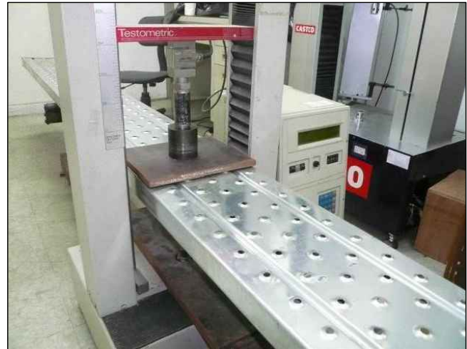
Testing of Planks at Support Interval 1,829 mm, Maximum Load P: 419 kg at deflection 62.02 mm
