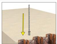
Step A1. Prepare to install the Sheet Pile Guard Post by inserting the claw vertically on the sheet pile wall.
