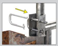
Step B2. insert the attached U-lock in the respective holes to hold the bracket in place; once U-lock is inserted, turn the latch flat to prevent from detaching.
