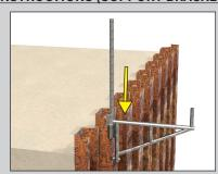
Step B1. Complete Steps A1-A2, attach a Cantilever Bracket to the top of the Sheet Pile Guard Post.
