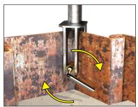
Step A2. Once the claw is clipped onto the sheet pile wall, secure Guard Post by turning the handle in the clockwise direction.
